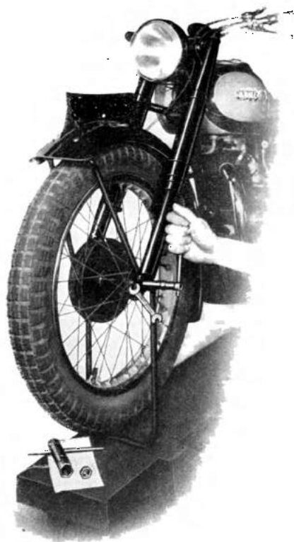
Fig. 18. Removing Front Wheel
